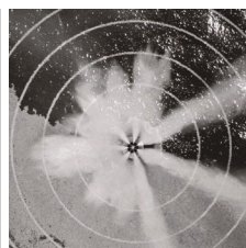
Poor injector spray pattern, from worn injector (photo taken with a microscope at nozzle point)
