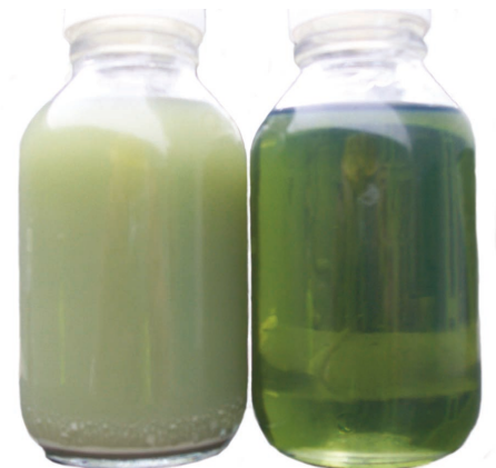
Industrial storage tank diesel fuel before and after CJC® Fuel Filtration
