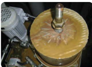
Dirty CJC® Filter Insert, saturated with dirt from the highly emulsified EAL oil. After filtration, the stern tube oil was free of water. Thus, risk of breakdown reduced!
