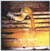
Water contamination on steel mill/ gear
